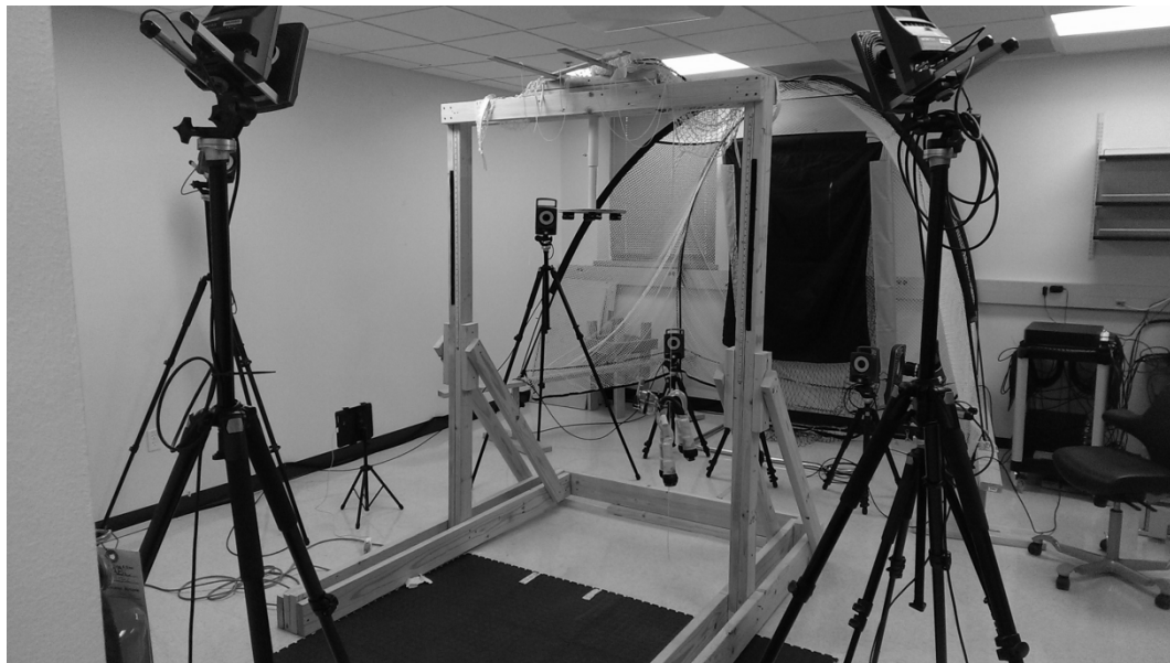
Figure 3. Eight-camera OMC system and simulated milking cluster attachment task setup.
